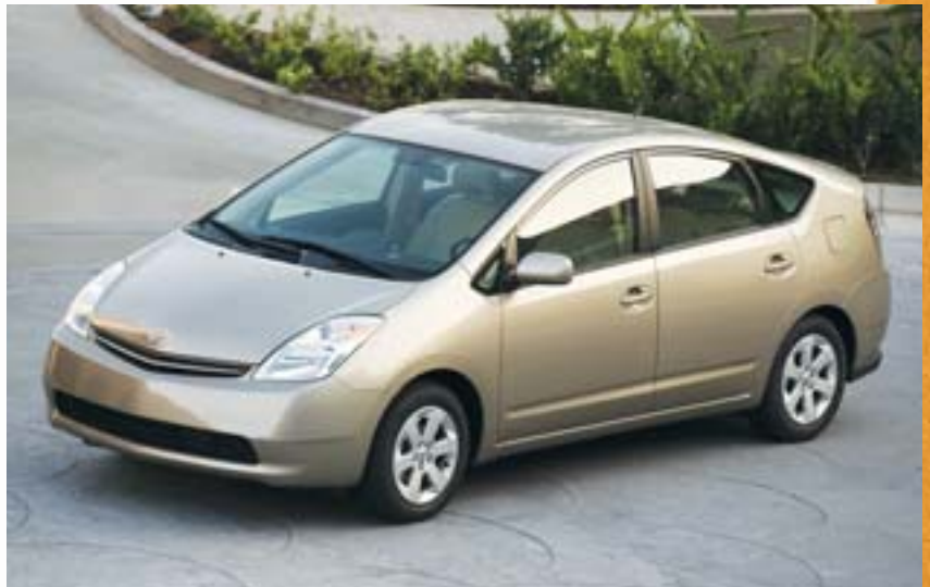
Prius, a hybrid vehicle from Toyota, saves fuel and cuts down on pollution by pairing a small engine with an electric motor.
